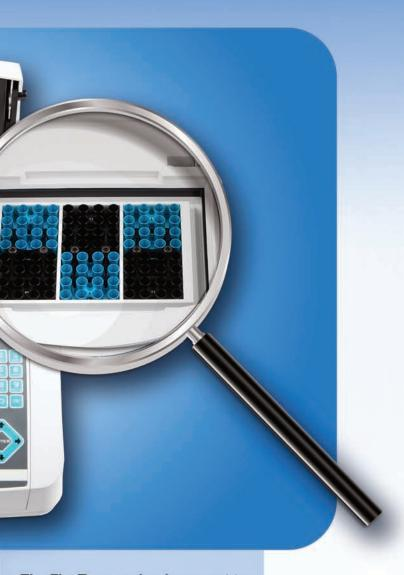
The FlexTemp technology provides a greater flexibility in approaching laboratory workflows. Because you can easily select annealing temperatures and because many primers work with common methods, you can run up to 16 wells of one primer at one temperature and 16 wells of another primer at another temperature during same run. The MultiGene OptiMax allows you to set 6 different temperature in each of the 4 x 4 well blocks. Maximum workflow flexibility.
